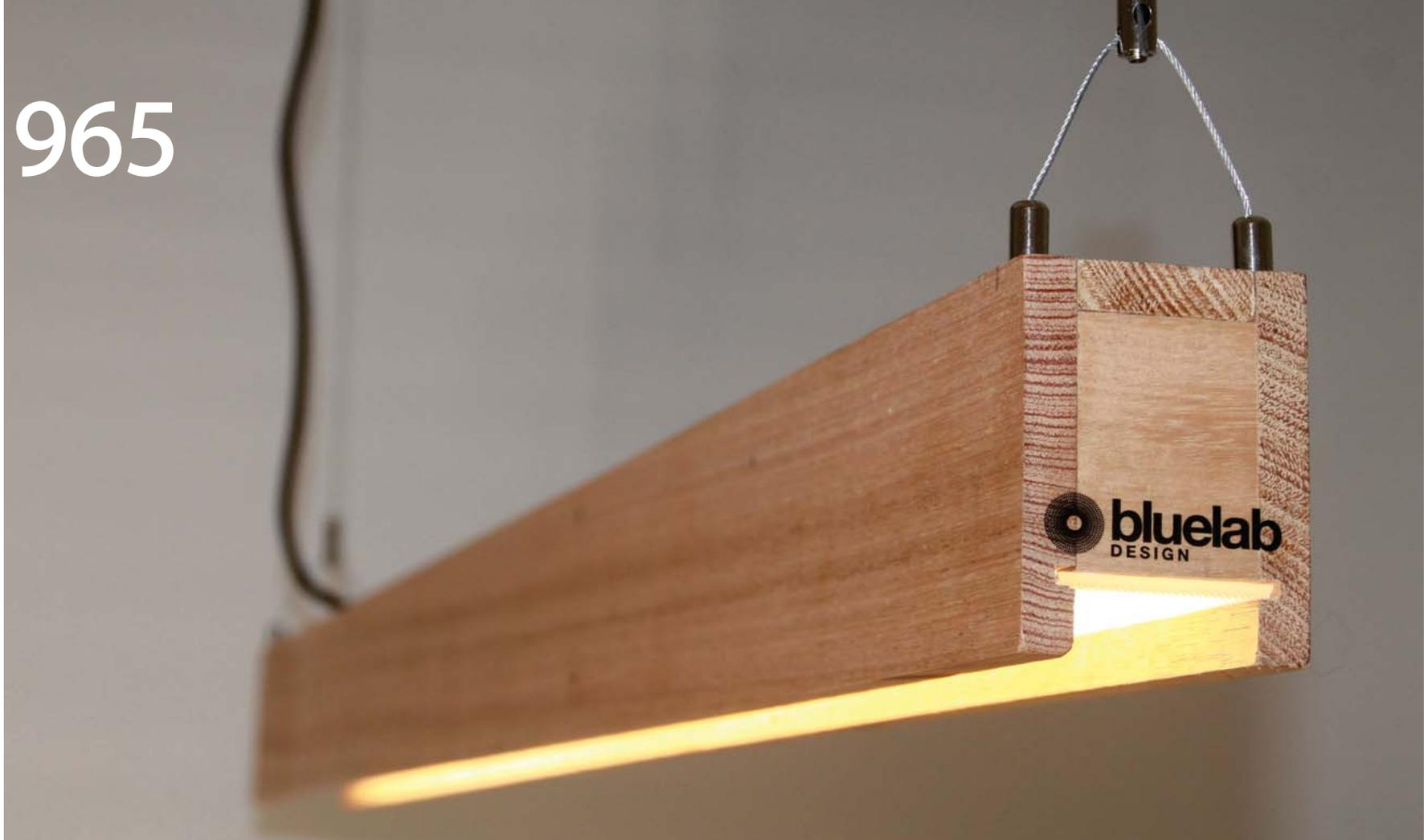
The Timber 965 can be crafted from any reclaimed, recycled or off the shelf hardwood. The regressed acrylic diffuser allows the light to showcase the natural grain. The fitting is supplied with a natural finish and can be stained and treated as required. Due to the led module used, the fitting is supplied in 560mm & 280mm increments.
