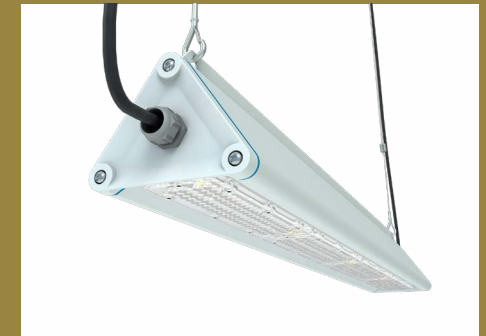
M25 cable gland with through-wiring (5 x 2,5mm 2 - L, PE, N, DA, DA).
