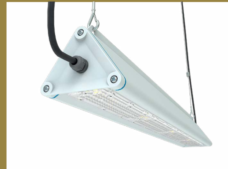
M20 cable gland with through-wiring (5 x 2,5mm 2 - L, PE, N, DA, DA).
