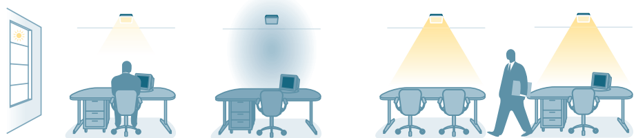
The light is controlled as a function of the incident daylight and movement.
