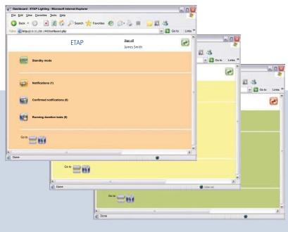
The window colours give you immediate recognition of the status of the luminaire's functionality.
